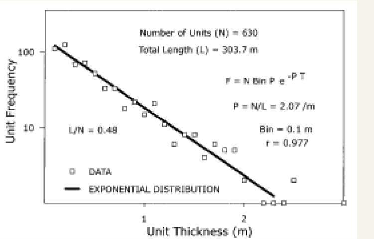
Data from Wilkinson et al. (1999) showing an exponential distribution of lithofacies thickness in Cambro-Ordovician carbonate strata outcropping in Wytheville, Virginia. The solid line is not a regression line but rather is theoretical exponential thicknessfrequency calculated for Poisson populations of several different lithofacies types with the same number of units and the same mean thickness as the outcrop data
