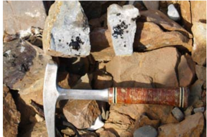
Figure 3. Basalt cobbles with live oil in vuggy pores found on a beach near a known seep locality along the South Nuussuaq coastline.
