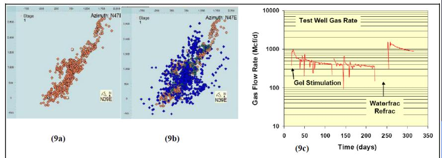
Figure 9 – Restimulation of Barnett well with slickwater is believed to contribute to increased fracture network complexity and superior gas production [Cipolla, 2005].
