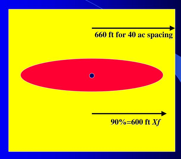
CE 100% if actual rate = rate with 600 ft infinite conductivity frac Absolute minimum-elliptical drainage not square
