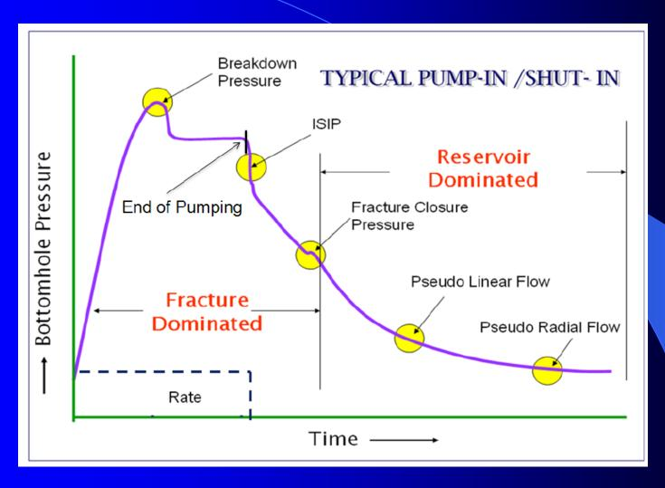
Small volume pumped enough to initiate a fracture
