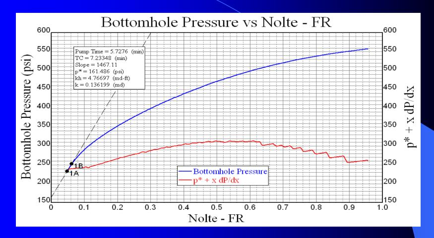
QC data with log-log plot to determine radial flow Small volume pump-ins do not require type curve analysis
