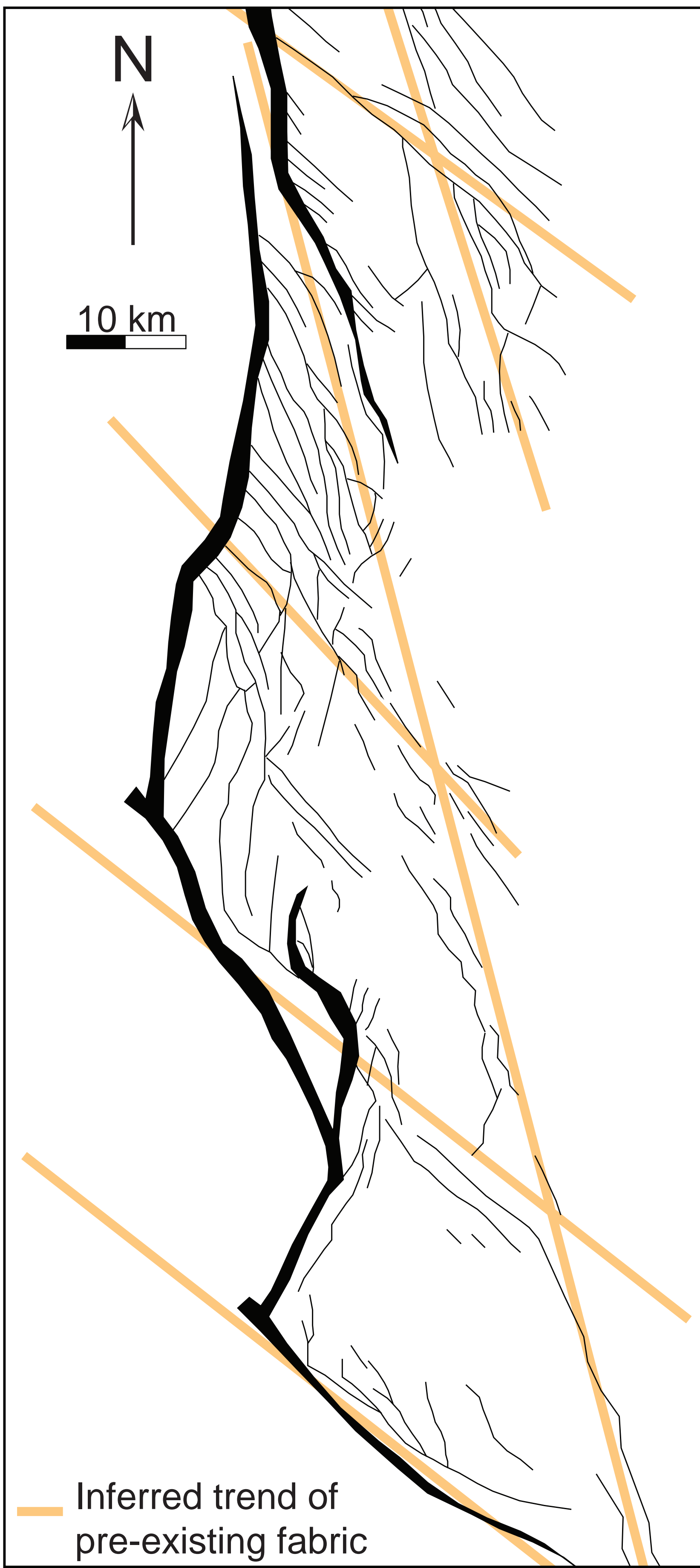
Map of the Pattani basin showing younger (Lower Miocene to recent), NNE- to NE-striking faults overlying older (Eocene-Oligocene), NNE- to N-striking faults. Map modified from Morley et al. (2004)
