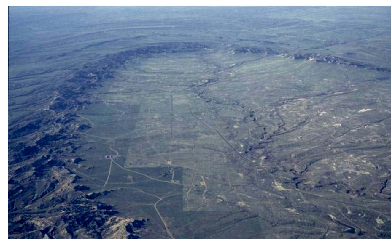
Aerial view above NPR-3 looking to the south. The Upper Cretaceous Parkman Sandstone highlights the asymmetric doubly-plunging anticline that forms Teapot Dome. Teapot Dome is cored by a west-verging basement reverse fault (Photo courtesy of John Lorenz).
