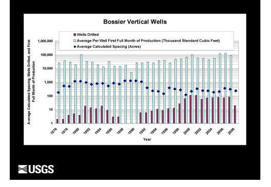
This figure compares trends in Bossier Formation well characteristics over time. Around 1990, there was an increase in drilling accompanied by a decrease in average well spacing and an increase in average first full month production. Data for 2008 are incomplete.
