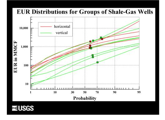
This is another way of comparing EUR distributions for analog groups of shale-gas wells. Squares represent the mean of each distribution. Note the large variation among groups. For example, the means for vertical well groups differ by greater than an order-of-magnitude. MMCF = millions of cubic feet.
