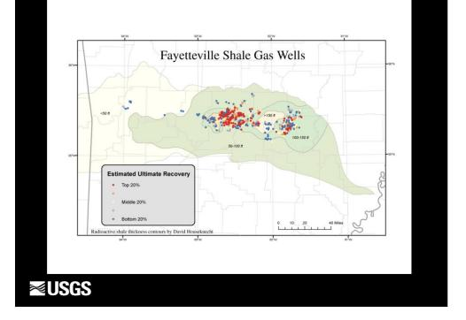
This map compares the well EURs of the previous map to the thickness of radioactive shale (as contoured by David Houseknecht, USGS). Note the moderate level of correlation between EUR and shale thickness.
