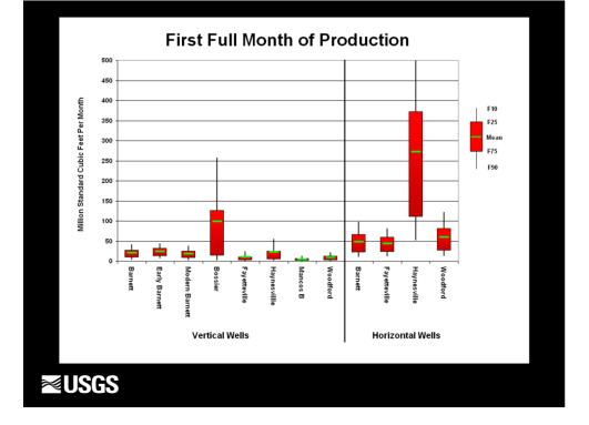
Comparison of several groups of shale-gas wells that could be used as analogs for assessments of data-poor areas. The box-and-whisker plots summarize the distributions of the first full month of production, which is commonly the highest monthly rate of production. Note the contrast between distributions of vertical and horizontal well productivities within the same formation. F90 denotes a 90 percent chance of at least the amount tabulated. Other fractiles are defined similarly.
