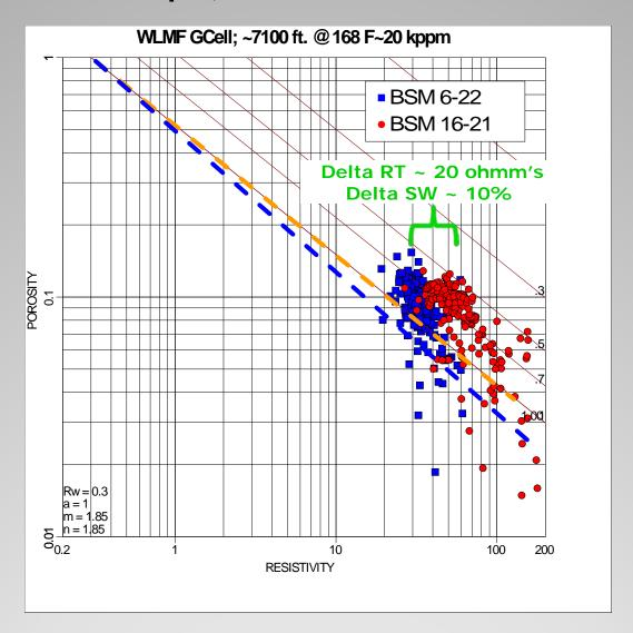
BSM 6-22 ~ Tested mostly water & Slight Gas BSM 16-21 ~ Tested 0.315 mmscfd
