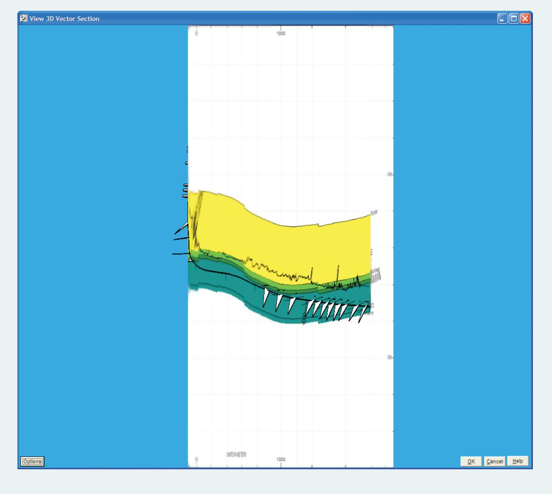
In Vector Sections, vectors point above or below the borehole perpendicular to dip with vector lengths in TST. Superimposed dips will parallel the horizon lines on the 3D vector section.
