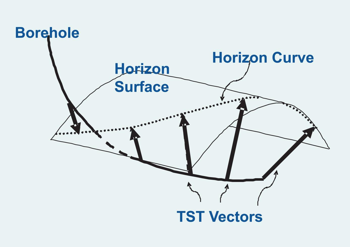
The vector is constructed such that if a given stratigraphic horizon is above the current point in the borehole, the vector points up and if the horizon is below that point, the vector points down.
