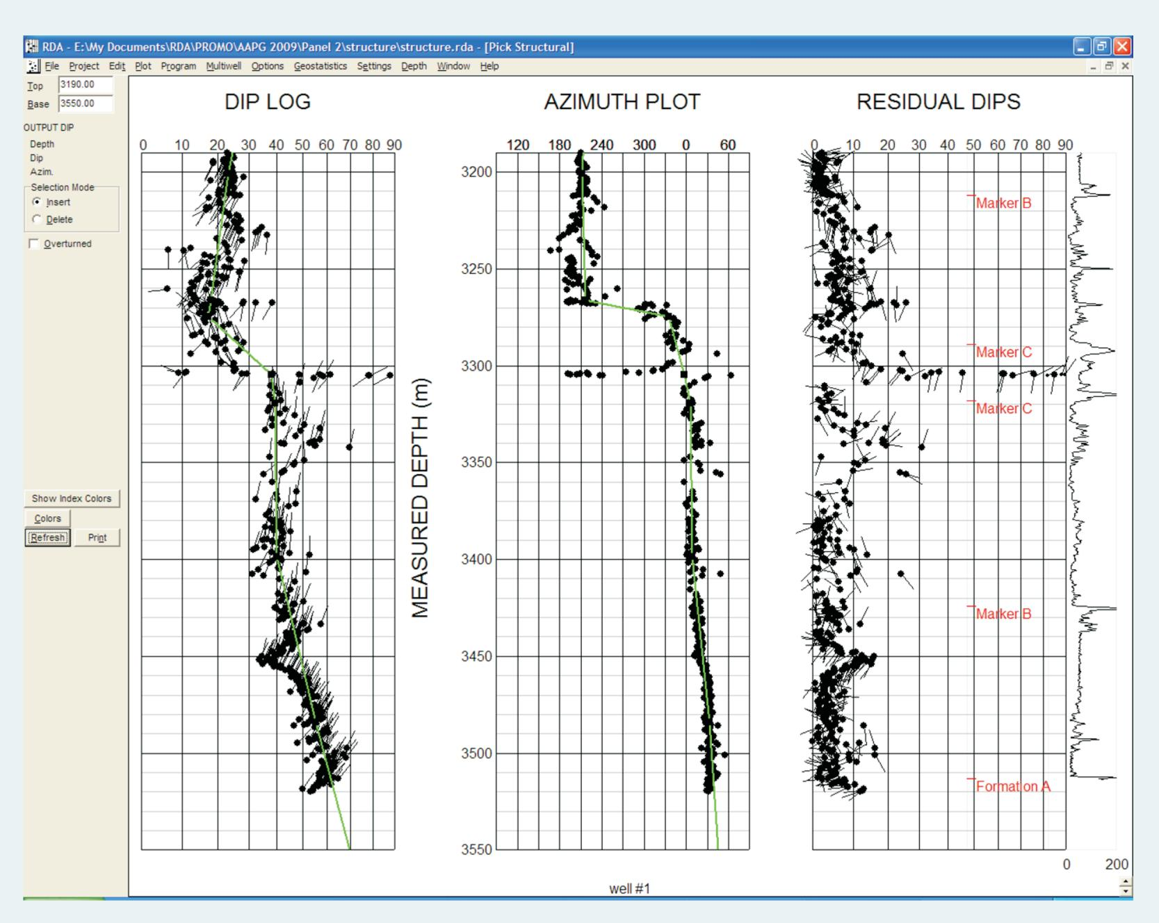
Structural dips are picked to smooth out the scatter inherent in dip data. This scatter is caused by variability within the dipscaused by measurement error, stratigraphically related variability, and minor structures.
