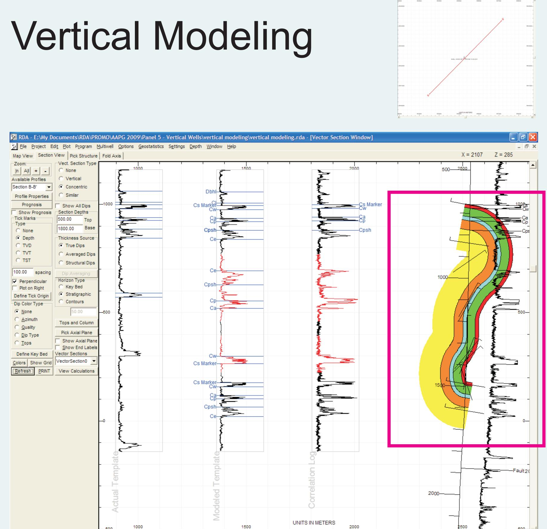
This well was modeled with only a gamma log and a deviation survey. On the left is an earlier, independently drawn cross section with essentially the same interpretation.
