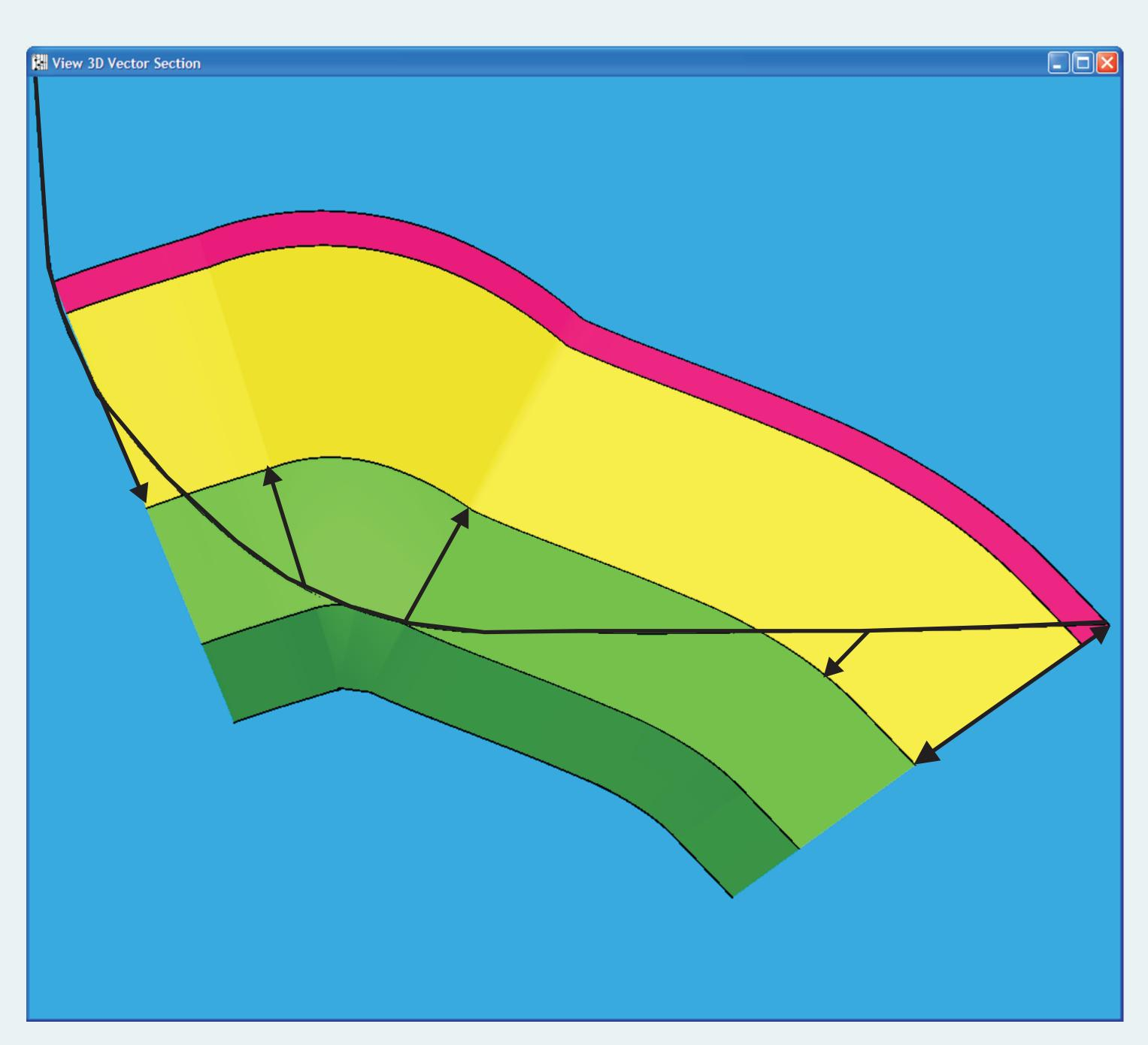
The structural dips that are picked on the left are used for the vector directions as well as for calculating TST for the vector lengths. In the downward-pointing vectors, the formation has a positive TST in relation to that point in the borehole. In the upward-pointing vectors, the TST is negative.
