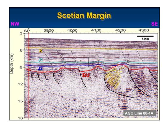
Highly-rotated fault blocks. Note the internal architecture with reflections expanding towards the fault strongly inferring a sedimentary origin. The Sinemurian age Breakup Unconformity is above the blocks that in turn confirms that the underlying crust cannot be oceanic and thus believed to be highly attenuated serpentinized mantle in the magnetic quite zone (MQZ).
