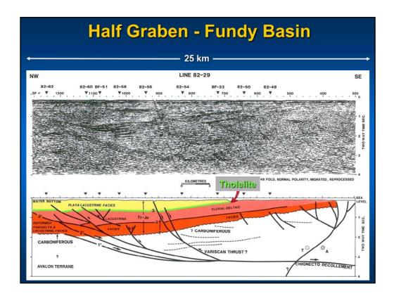
The half graben architecture and general stratigraphy of the continental Chignecto Subbasin is similar to that of the Tupi depocentre but without the salt. Salt-capped half grabens may though exist deeper in the Scotian Basin (e.g. Orhpeus Graben).
