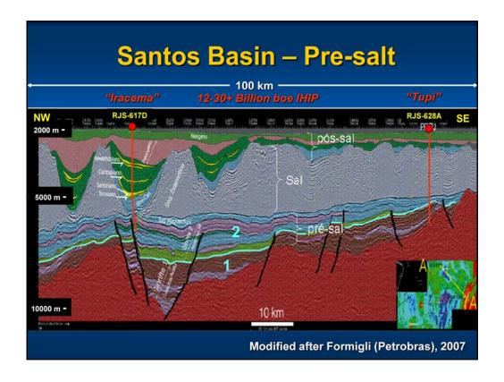
Guaratiba Formation – lacustrine siliciclastics and limestones – coquinas (reservoirs), lacustrine shales (source). Lower succession fluvial sandstones, conglomerates and playa mudstones. The Iracema and Tupi discoveries are estimated to be a single accumulation containing 12-30+ billion BOE initial hydrocarbons in place (IHIP).
