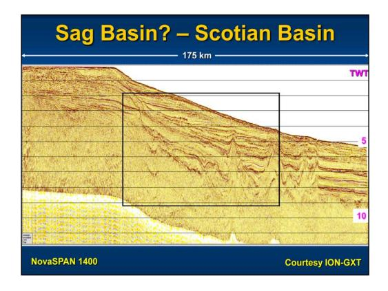
Example of a portion of the southwestern Scotian Basin that may have an underlying sag basin. Thick overlying Tertiary to Jurassic successions are considered to be masking a series of possibly interconnected, deeper basement features that acted as loci for Argo formation (Hettangian) salt deposition. The black outline is the area shown on the next slide.
