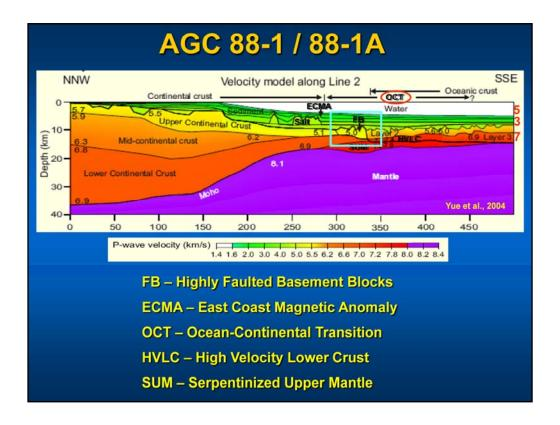
Note thicknesses of water, sediments and crust. Blue box outlines the area illustrated in the seismic line of the next slide.
