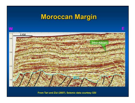
Highly Rotated Fault Blocks on the Moroccan conjugate margin. Note their landward-dipping character and internal geometries indicative of concurrent sedimentation extensional faulting. Tertiary to early Jurassic successions overly the HRFBs.
