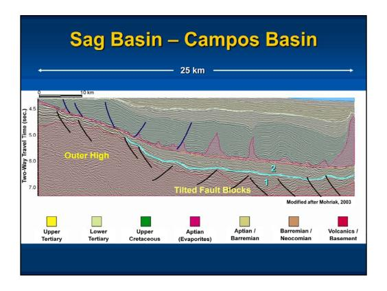
Blue line indicates two syn-rift packages; the lower fluvial and alluvial, the upper fluvial and lacustrine.
