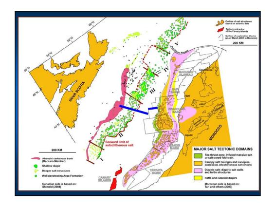
Salt and basin locations, Nova Scotian and Moroccan margins. Blue lines indicate the location of two conjugate seismic lines that reveal the presence of Highly-Rotated Fault Blocks (HRFB) on interpreted attenuated mantle, not oceanic, crust.
