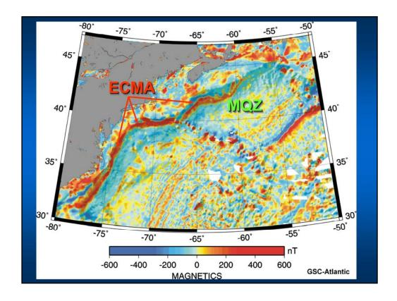
ECMA = East Coast Magnetic Anomaly; MQZ = Magnetic Quiet Zone. The Highly Rotated Fault Block (HRFB) features are located on the MQZ that was originally interpreted as oceanic crust but is now believed to be highly attenuated serpentinized upper mantle.
