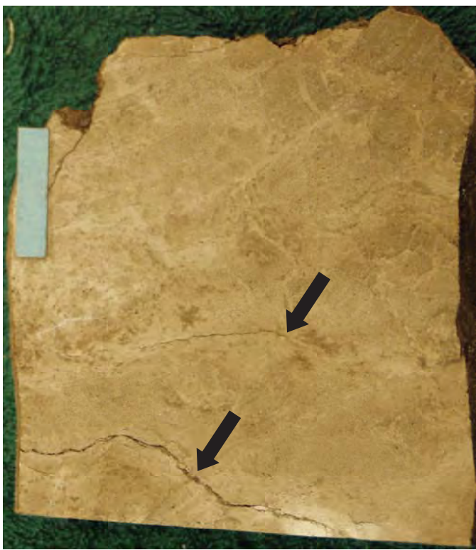
Core slab of stylolitic (arrows) micro-porous tripolite. Scale 1". General Atlantic #1-A Tjaden, 4372 ft.
