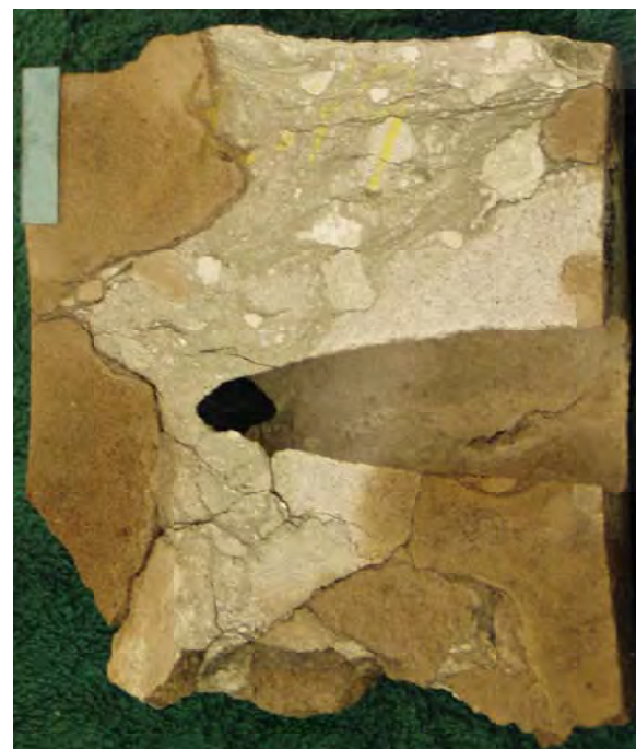
Core slab of brecciated spiculitic tripolite. General Atlantic #1-A Tjaden, 4348 ft.
