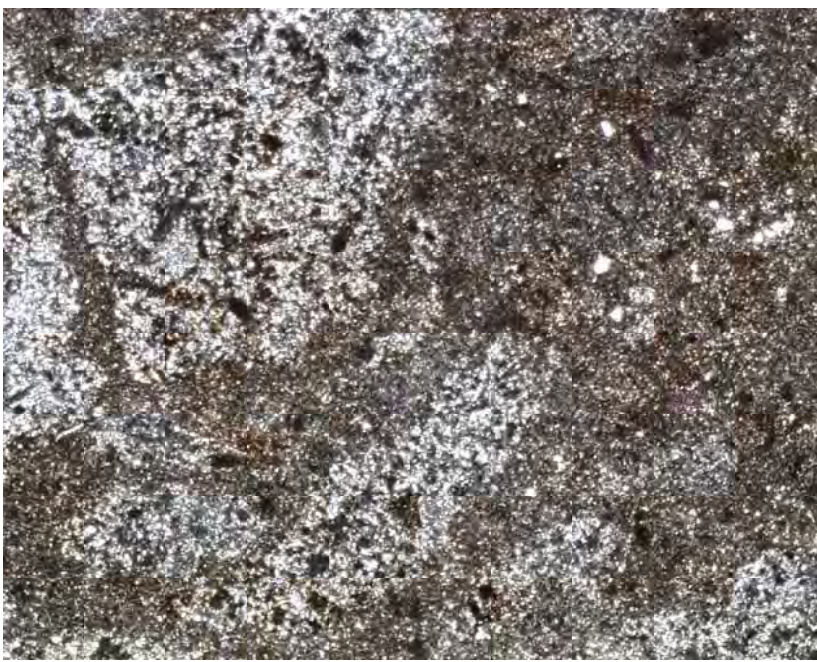
Thin-section photomicrograph of micro-porous tripolite; 40x magnification, crossed nicols. General Atlantic #1-A Tjaden, 4377 ft.
