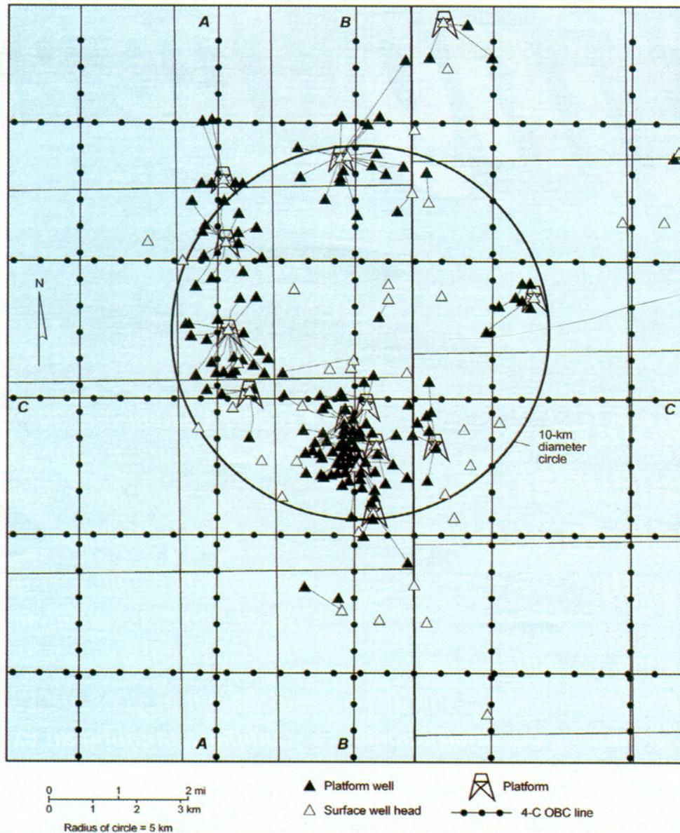
**Figure 2. 4-C OBC data acquisition across one specific area of production congestion. Note how close OBC lines AA, BB, and CC are to many of the production facilities.**
