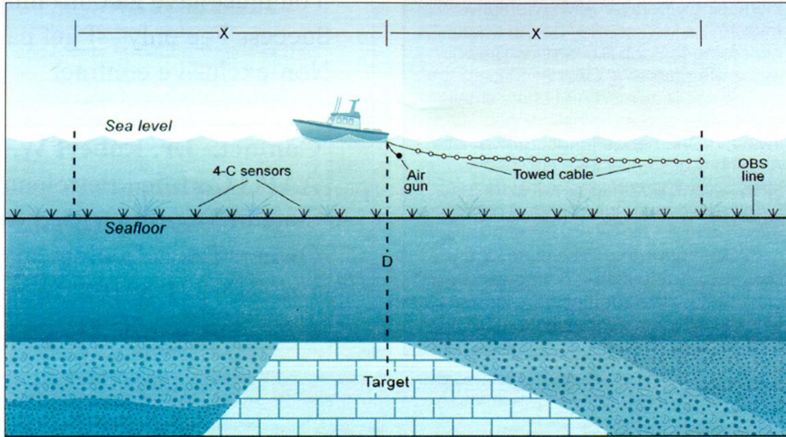
Figure 1. To image a target at depth  $D$ , the distance  $X$  from the source to the farthest receiver should equal or exceed  $D$ . Two options are shown for acquiring long-offset marine seismic data: super-long towed-cable technology and stationary ocean-bottom sensors (OBS) deployed on the seafloor. Seafloor sensors can be deployed as individual sensor packages with self-contained data storage or as long ocean-bottom-cable (OBC) linked to a recording boat.
