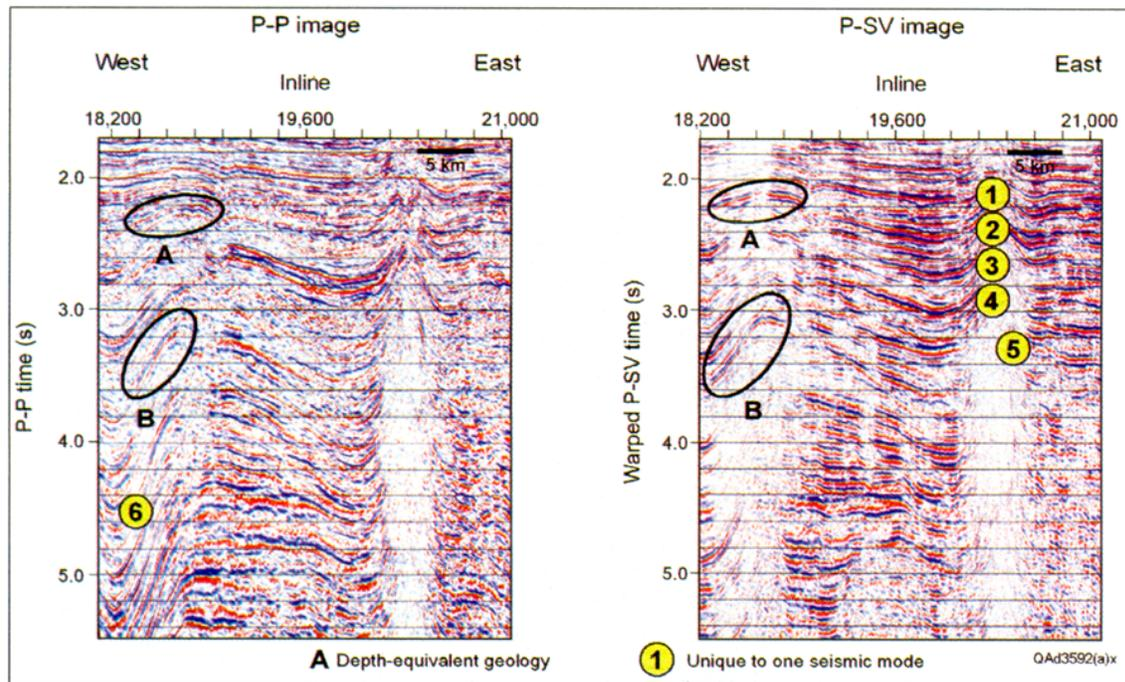
Figure 3. Comparison of deep, depth-equivalent P-P and P-SV data windows across an area of congested production facilities in the Gulf of Mexico.
