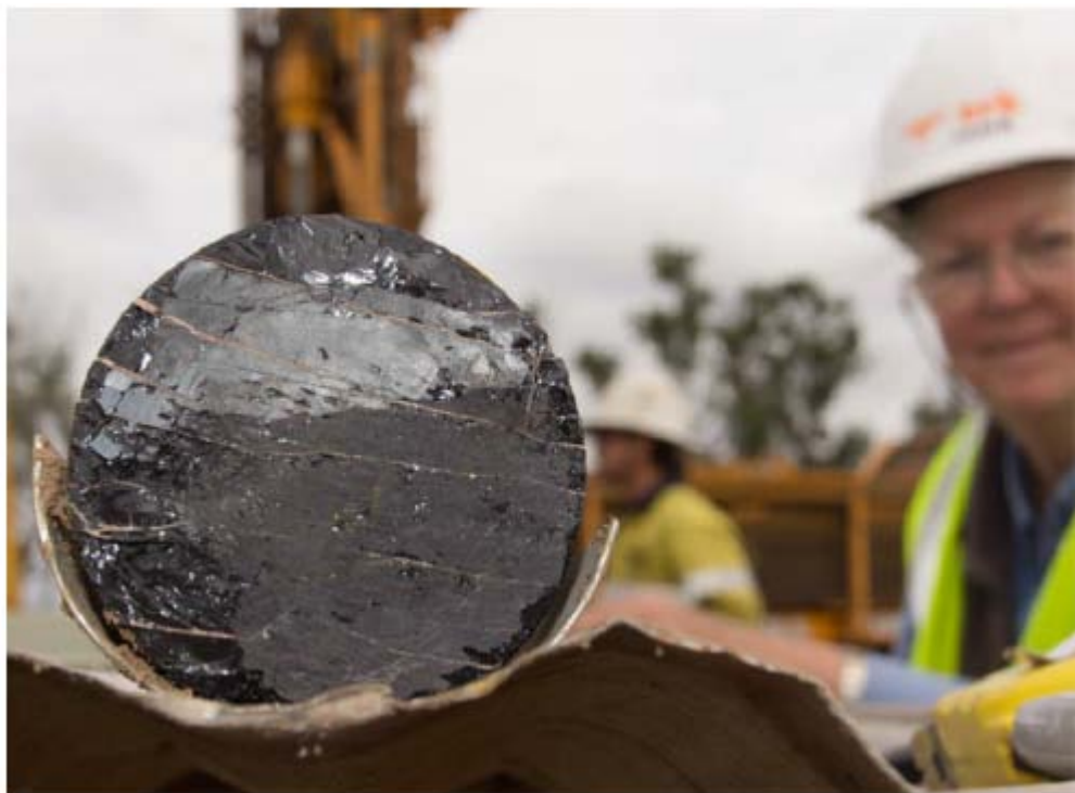
Figure 3. Calcite cleat infill in southern Bowen Basin Bandanna (Rangal) coal.
