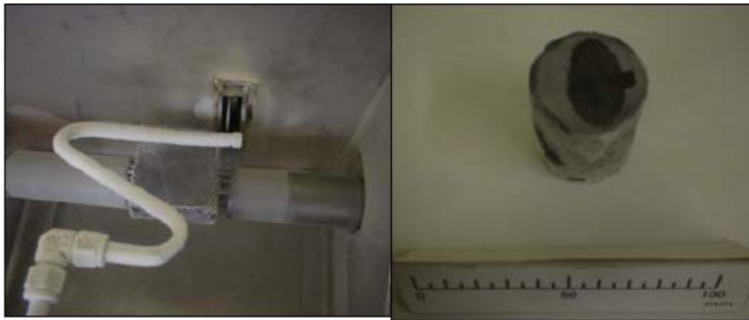
Figure 3. Oil sands sample plug; (a) Trimming and (b) Oil Sand Plug.
