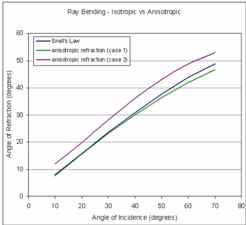
Figure 1. Diagram showing the complex relationship between the angle of incidence and refraction when dipping anisotropy is present.
