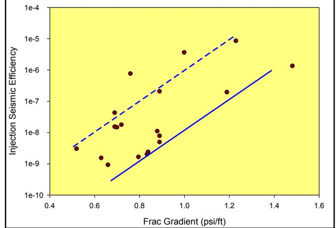
**Figure 1. Plot of seismic injection efficiency versus frac gradient (after Maxwell et al., 2009). Solid blue curve represents a low SIE “conservative” trend and dashed a high SIE trend.**
