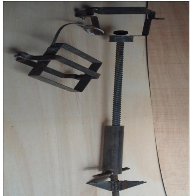
Figure 3: Ground anchor for securing RAUs
