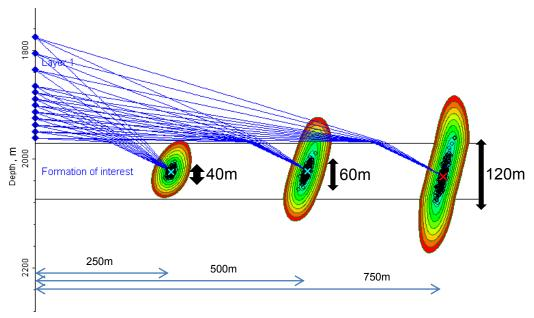
Figure 2: Monte Carlo solutions for each of the theoretical events (X's) (200 trials with Traveltime Error of 2ms) placed in 250m increments away from the extended 12 level toolstring placed above the zone of interest
