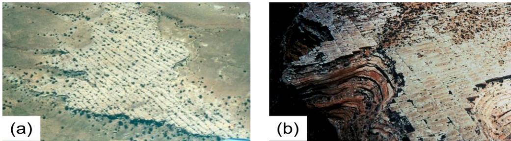
Figure 1: Aerial photos of fracture outcrop. (a) mono-oriented vertical extension fractures, San Juan Basin; (b) two sets of vertical extension fractures in sandstone, Cedar Mesa Fm. Photos courtesy of Scott Cooper and John Lorenz.
