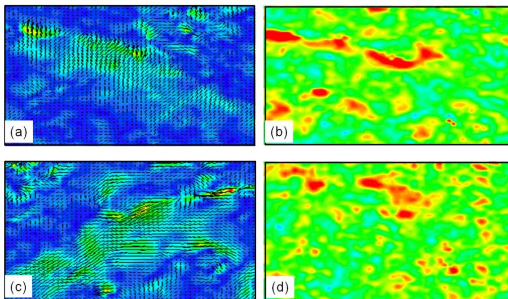
Figure 2: VVAZ/AVAZ comparison. (a) VVAZ fracture intensity (colour) with orientation vector overlay for upper Devonian shale; (b) AVAZ fracture intensity at top upper Devonian; (c) VVAZ fracture intensity for middle Devonian carbonate; (d) AVAZ fracture intensity at base upper Devonian.
