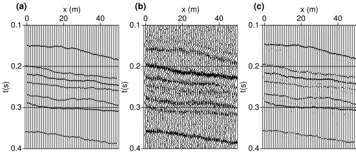
**Figure 1** Synthetic data example. (a) Original reflectivity series utilized to test the proposed blind deconvolution algorithm. (b) Seismic data modelled by convolution of the reflectivity with a Ricker wavelet with phase rotation  $60^{\circ}$ . The data were also contaminated with noise (SNR = 6.0). (c) Sparse reflectivity series obtained by the proposed blind deconvolution method.
