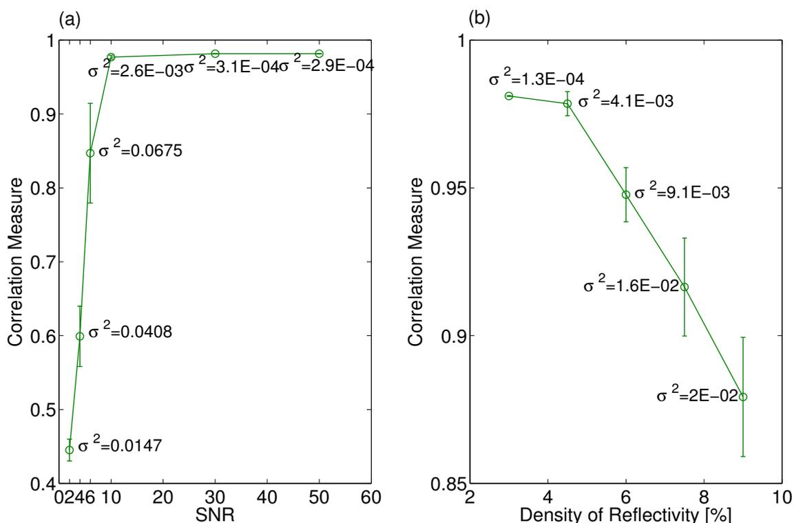
**Figure 3** The normalized correlation between the estimated and true wavelet for different (a) SNRs and (b) density of reflectors (the density measures the percentage of non-zero coefficients of the reflectivity series).
