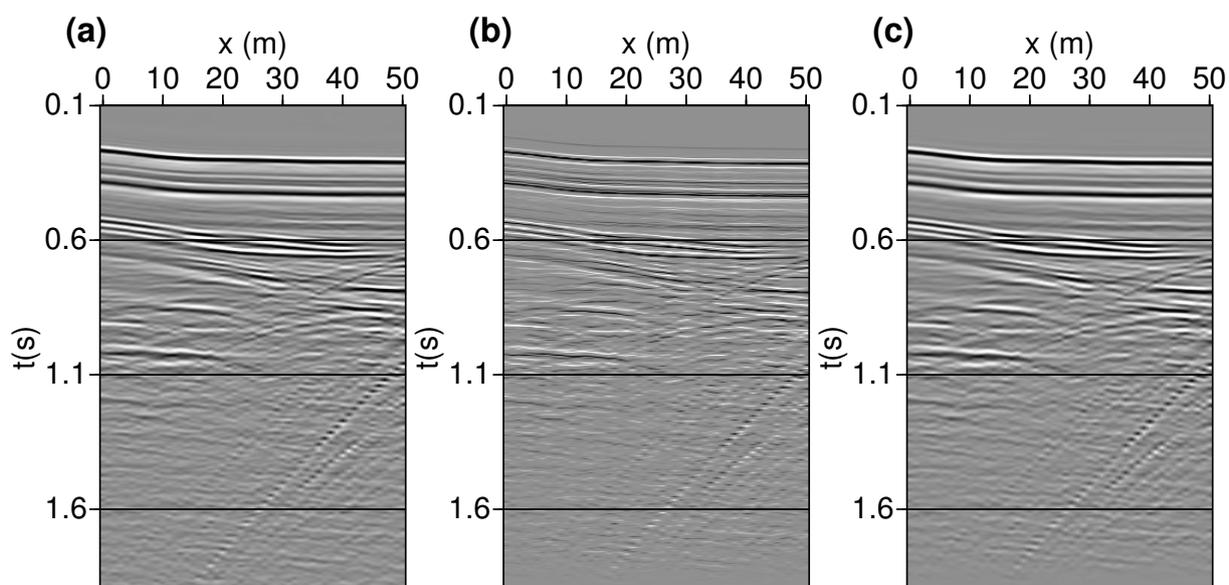
**Figure 4** Real data example. (a) A window of the Mississippi Canyon marine seismic data. (b) Reflectivity series estimated via the proposed algorithm. (c) Seismic data after convolution of the estimated reflectivity with the estimated wavelet.
