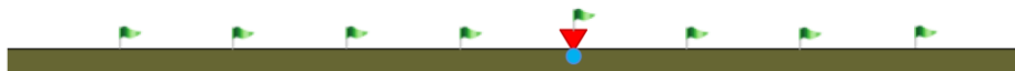
Figure: 1. A 2D model including one source (red triangle) on the top of a scatterpoint (blue circle) and eight receivers (flags) on the earth surface.
