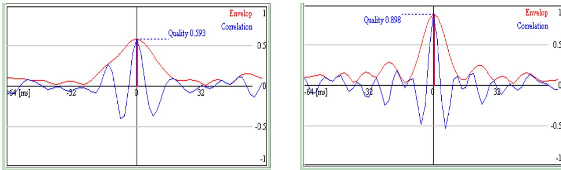
The plot below is the seismic data before and after the match filter demonstrating the enhanced resolution achieved by normalizing the the high frequency and aligning frequencies at zero phase with the match filter.
