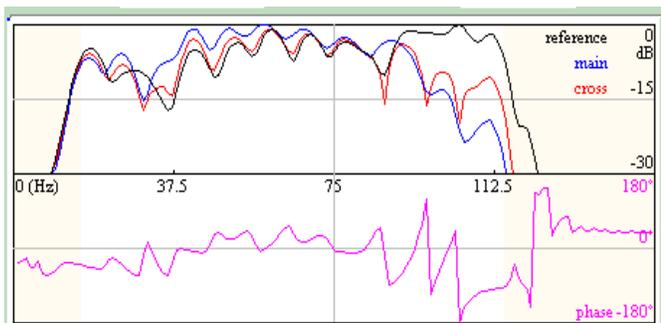
It is clear that the seismic trace amplitude spectrum (main) in blue does in fact contain the requisite 100 Hz energy but this is down by 15dB as a result of the phase distortion above the 85 Hz level as depicted on the phase plot.
