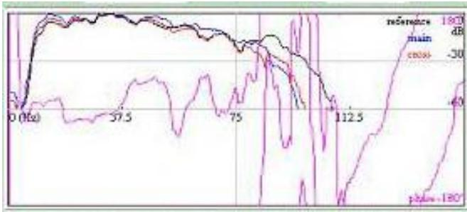
This example shows the useable limit of the frequency to be around 85 Hz demonstrating that the frequency above 85 Hz is not useable.
