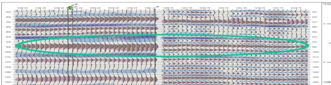
Since a match filter operator only changes the wavelet a properly derived match filter operator should theoretically be just as applicable to gather traces as to stack data. This is easily demonstrated by the gathers from this dataset with and without the same Match Filter Operator applied.
