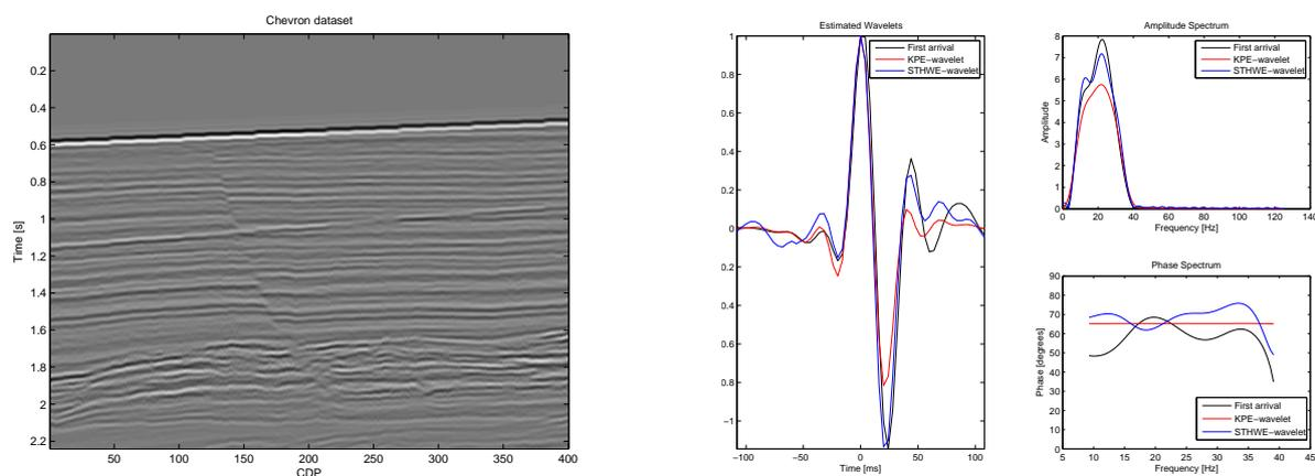
**Figure 1** Dataset used to compute the wavelet (left). Center plot shows the estimated wavelets, in black is the first arrival (FA), the KPE method (red) and the short-time homomorphic method (blue). In the upper right panel the three amplitude spectrums are plotted and in the right bottom their corresponding phase spectra.
