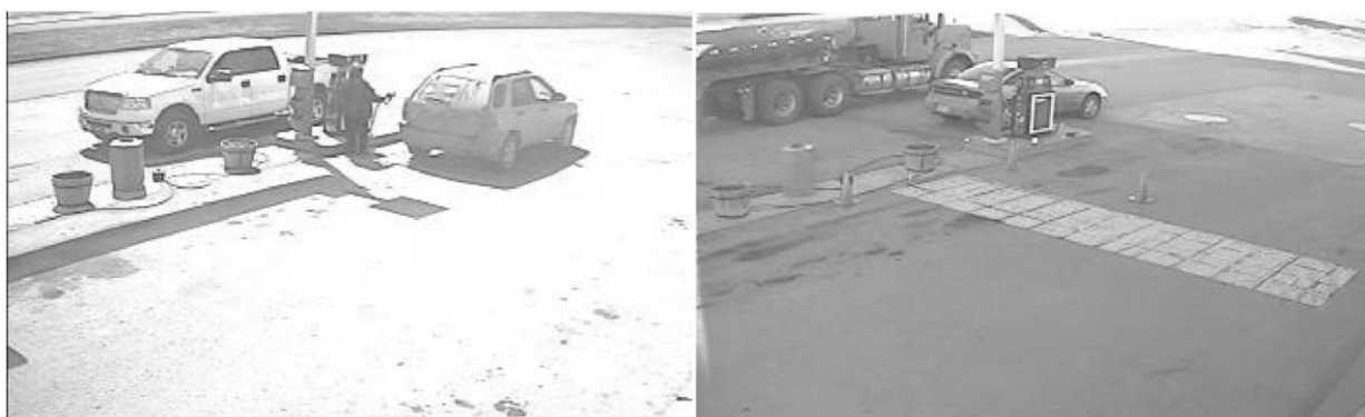
Figure 1: Left : Security camera frame from Lashburn, SK, showing the shadows cast by the fireball; in this case notable shadows are being cast by the light fixtures above the gas pumps. Right : Calibration image taken through the security camera, a regular grid pattern was used to measure the shadow positions relative to the object casting the shadow.
