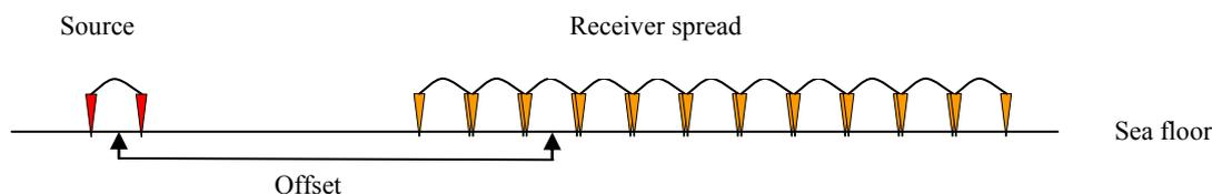
**Figure 1** Acquisition geometry for OBC transient EM surveying.
