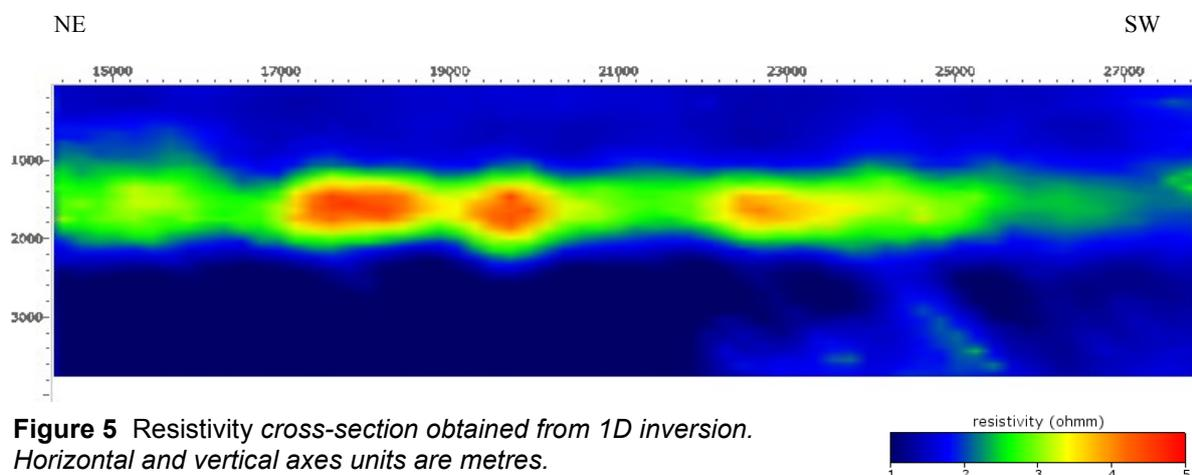
**Figure 5** Resistivity cross-section obtained from 1D inversion. Horizontal and vertical axes units are metres.
