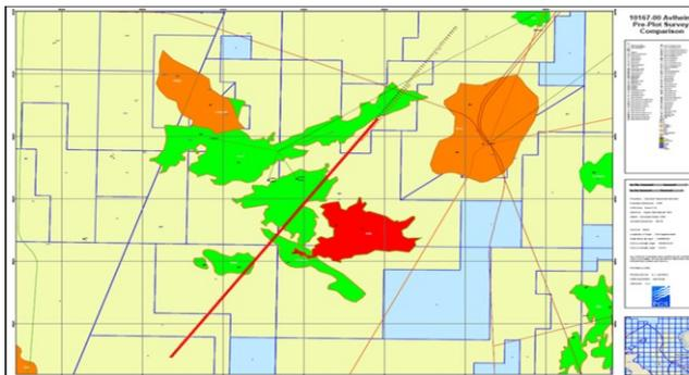
**Figure 2** Transient EM survey profile line (red) across the Alvhheim field.
