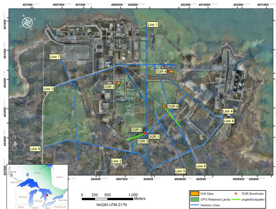
Figure 1: Bruce nuclear site showing 2-D seismic reflection survey lines, vertical (DGR-1, DGR-2, DGR-3, DGR-4) and angled (DGR-5, DGR-6) boreholes surrounding the proposed repository footprint.
