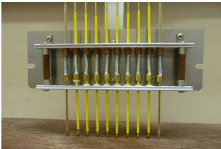
Figure 2: A linear array of ten piezopin transducers. Adjacent transducers are separated by 10 mm. In this array, the two end transducers are used as receivers; the eight transducers in the middle are used as transmitters.
