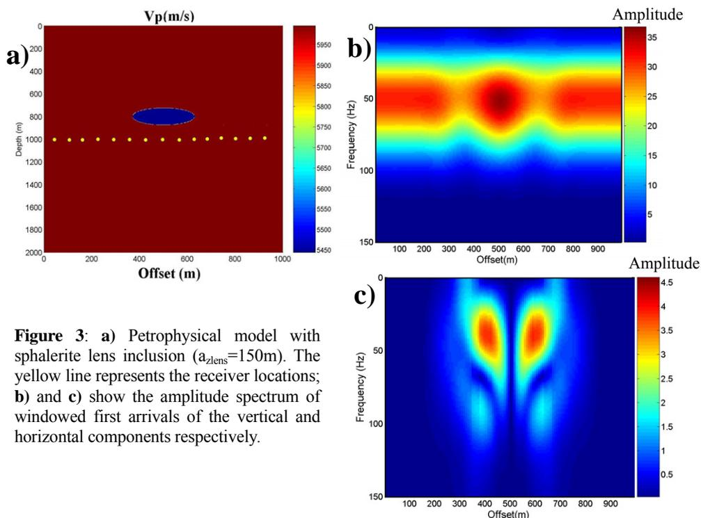
**Figure 3:** a) Petrophysical model with sphalerite lens inclusion ( $a_{\text{lens}}=150\text{m}$ ). The yellow line represents the receiver locations; b) and c) show the amplitude spectrum of windowed first arrivals of the vertical and horizontal components respectively.
