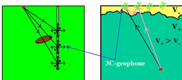
**Figure 1:** Geometry illustrating scattering by limited target (left panel), and the case of overburden (right panel, large reflection coefficient R).
