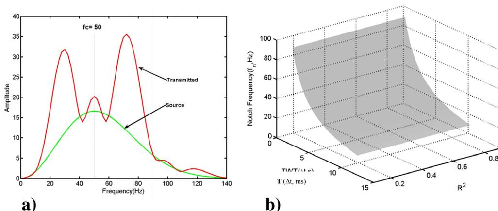
**Figure 2: a)** Amplitude spectrum of transmitted energy in two-layered medium illustrating the overburden effect: gneiss (5933 m/s, 2722 kg/m<sup>3</sup>) and clay overburden (2000m/s, 2000 kg/m<sup>3</sup>, 20m thick). Analysis is based on normal incidence. The transmitted trace consists of the direct arrival and two multiples.
