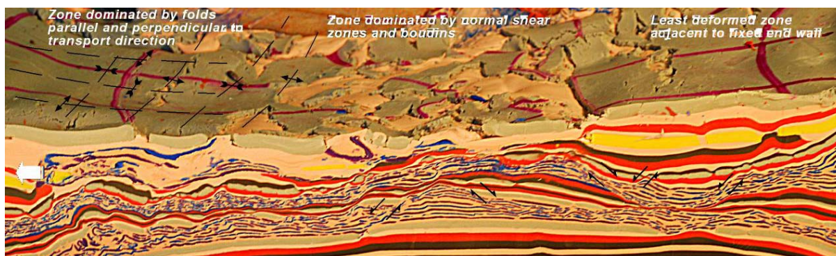
Figure 5: Oblique view of upper surface and vertical cut through a model simulating collapse between convergent lateral ramps showing changes from extensional to contractional deformation similar to that found in some deltas.
