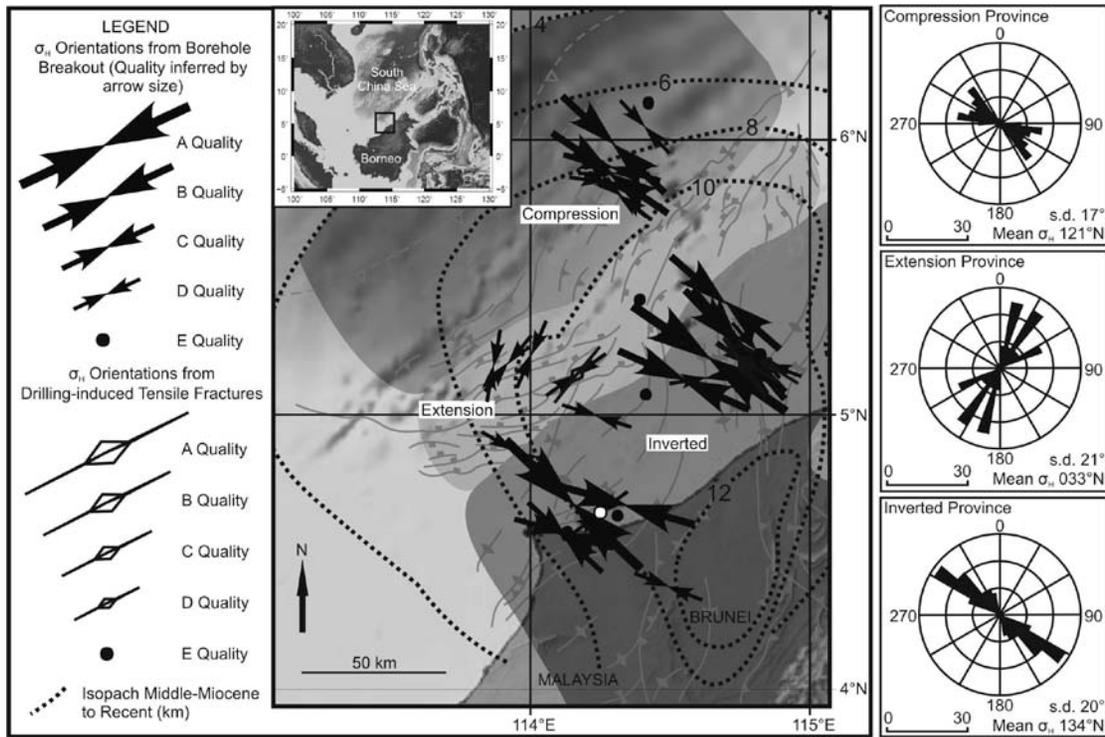
**Map of the Baram Delta System, NW Borneo, demonstrating the location and extent of the three neotectonic provinces and the maximum horizontal stress orientations that have been determined using image logs from 56 petroleum wells.**
