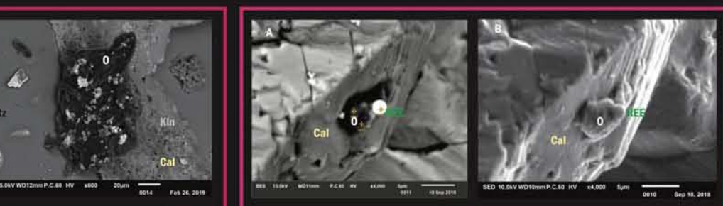
Figure 17: Examples of bitumen particles A) Bitumen with sylvite on quartz, can be seen as the dark spot on grain D from Figure 7. B) Bitumen with sylvite, halite, and siderite on kaolinite included calcite like that seen in Figure 9A, all on top of a quartz euhedra. C) Cubic microcubes of halite precipitating from the bitumen particle in B.
