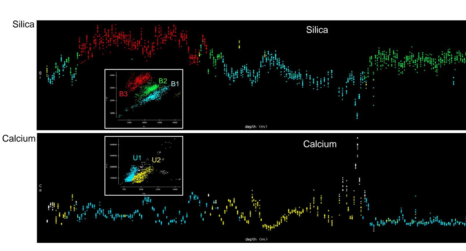
Continuous XRF analysis of cuttings delivers cheap and reliable results to recognize stratigraphical units and diagenetic alteration allowing for optimal frac design
