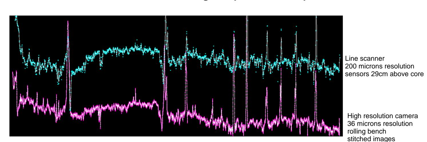
Outstanding match between shades of grey by two laboratories and two completely different technologies
