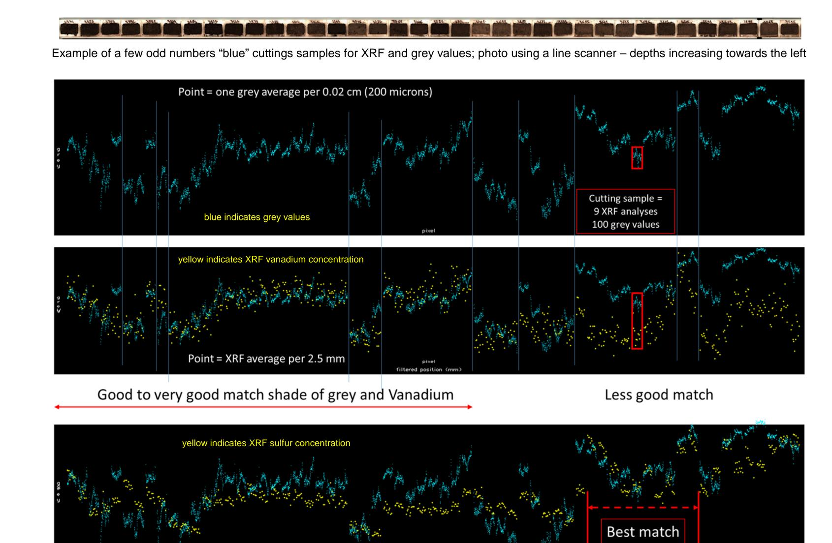
Shades of grey every 200 microns have been compared to some XF elements in order to identify different types of organic matter (TOC).
