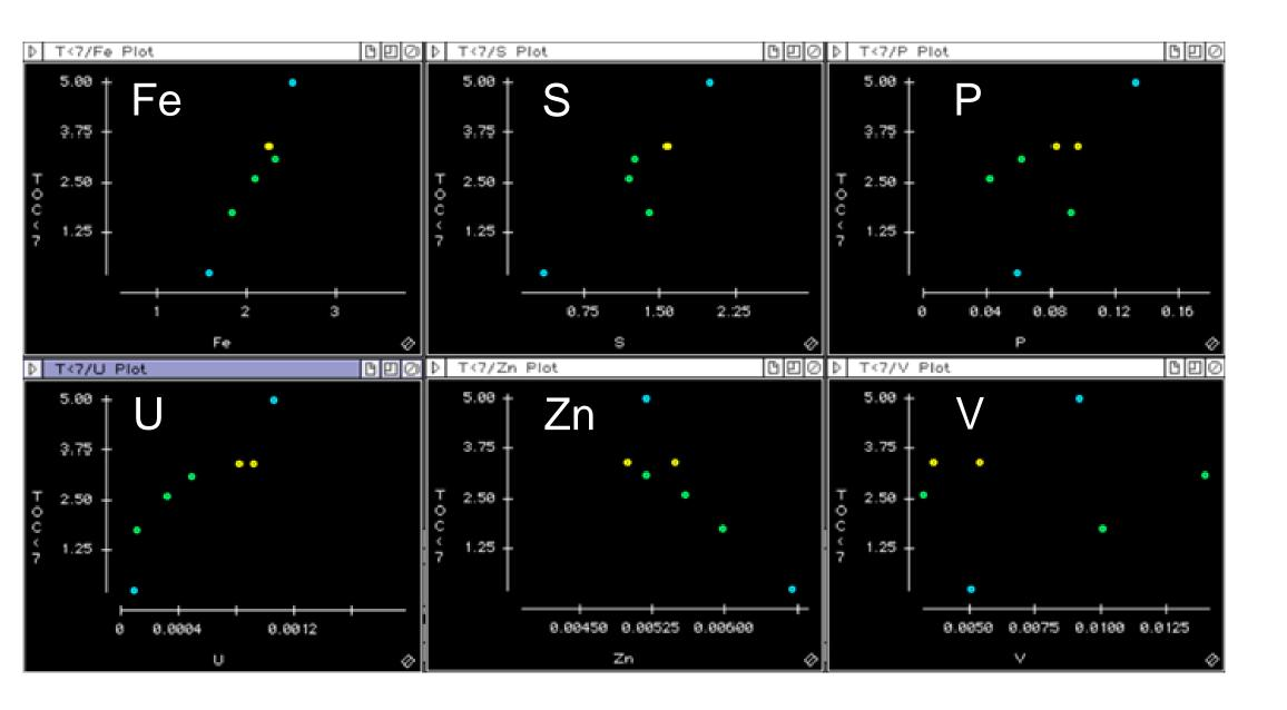
The colors indicate three different laboratories that measured the TOC content from core material. The well is located in the East Duvernay Basin. Note the near perfect relationship of TOC with Iron.
