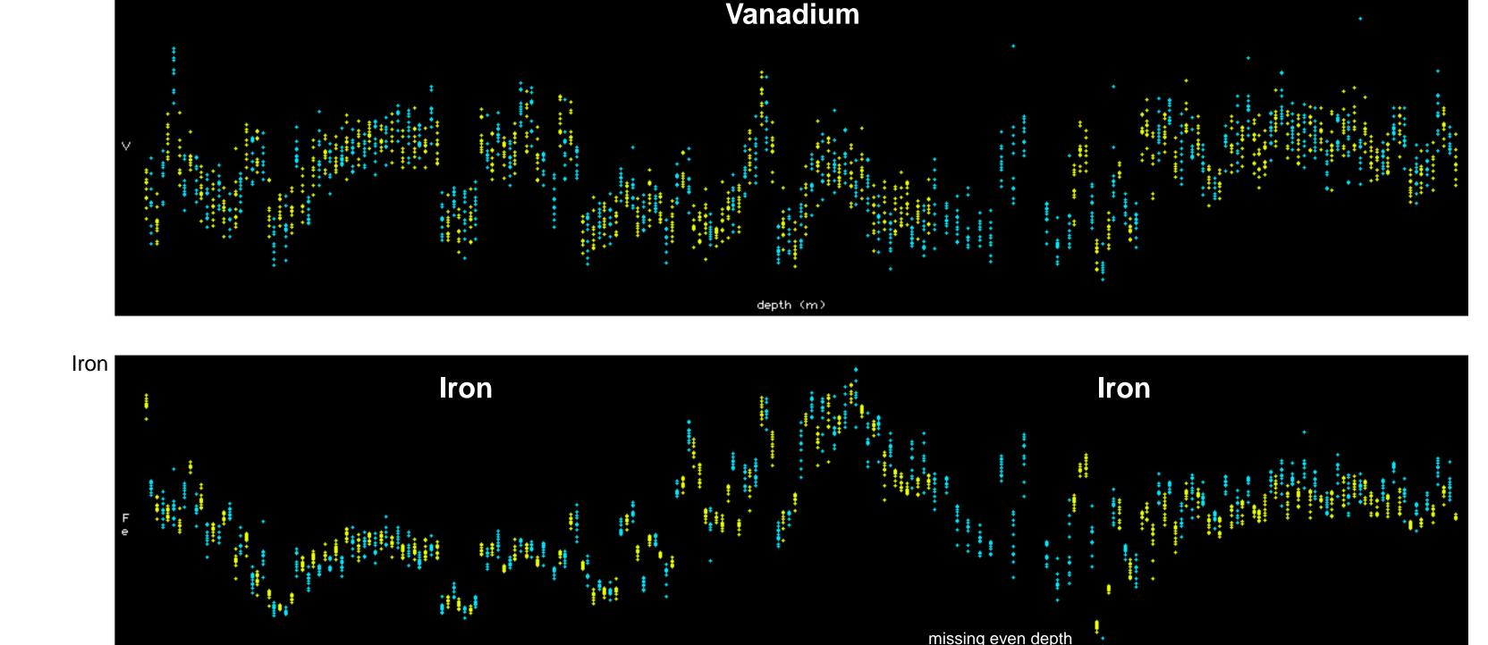
Four sets of cuttings have been analyzed with the ITRAX XRF device; samples every 5 m (same color 10 m)
