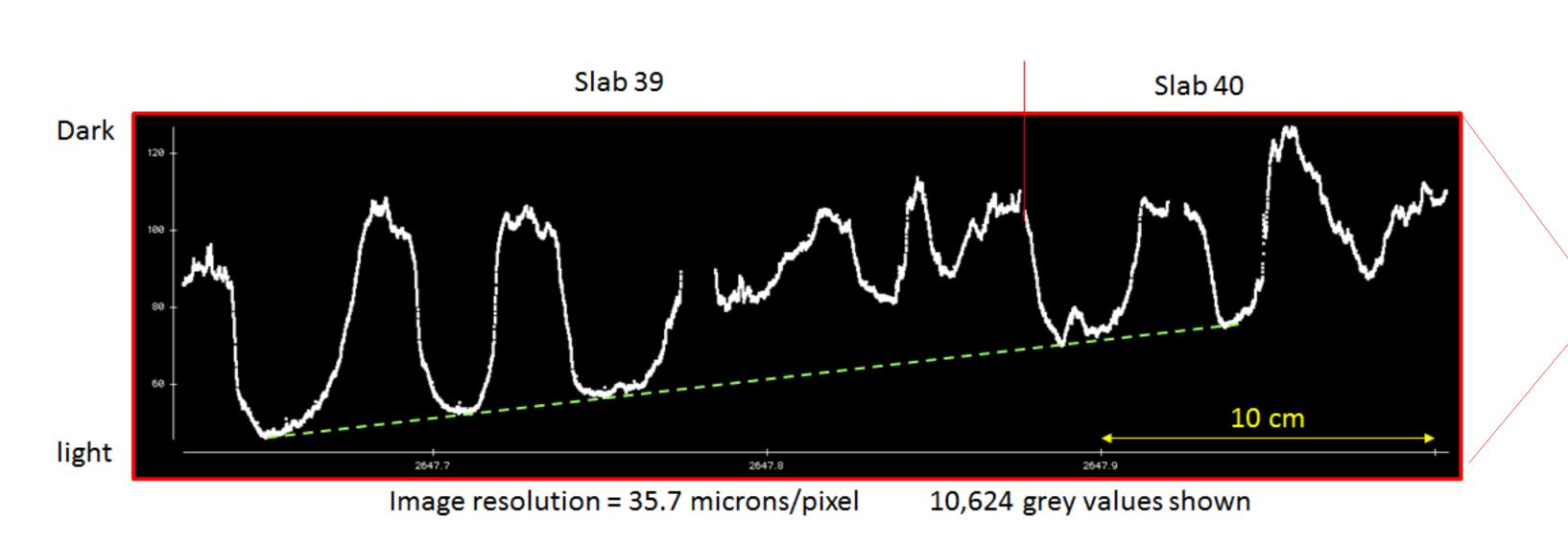
Outstanding trend showing lightening upward carbonate on an interval 3metre thick Note the perfect transition in shades of grey between Slab 39 and slab 40
