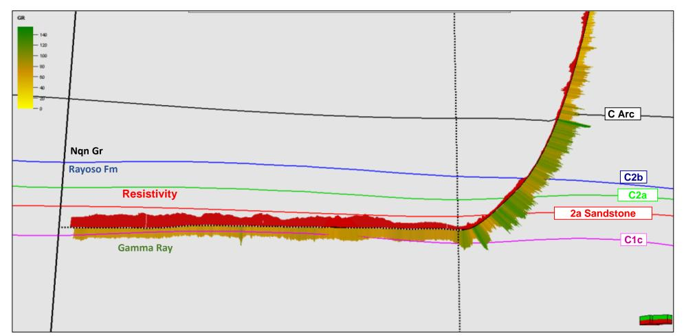
Use of horizontal wells resulted a good development strategy because of the reservoir areal extent, the good petrophysical properties of Cycle 2a and the reduced oil halo due to the gas cap.
