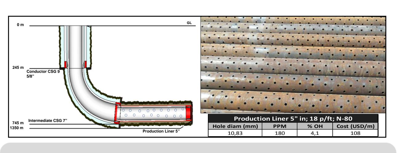
Well architecture was designed to satisfy the reservoir, production and drilling requirements in order to optimize production and costs reduction. Before the drilling campaign started, a geosteering model was prepared for each proposed well using resistivity as the input property.
