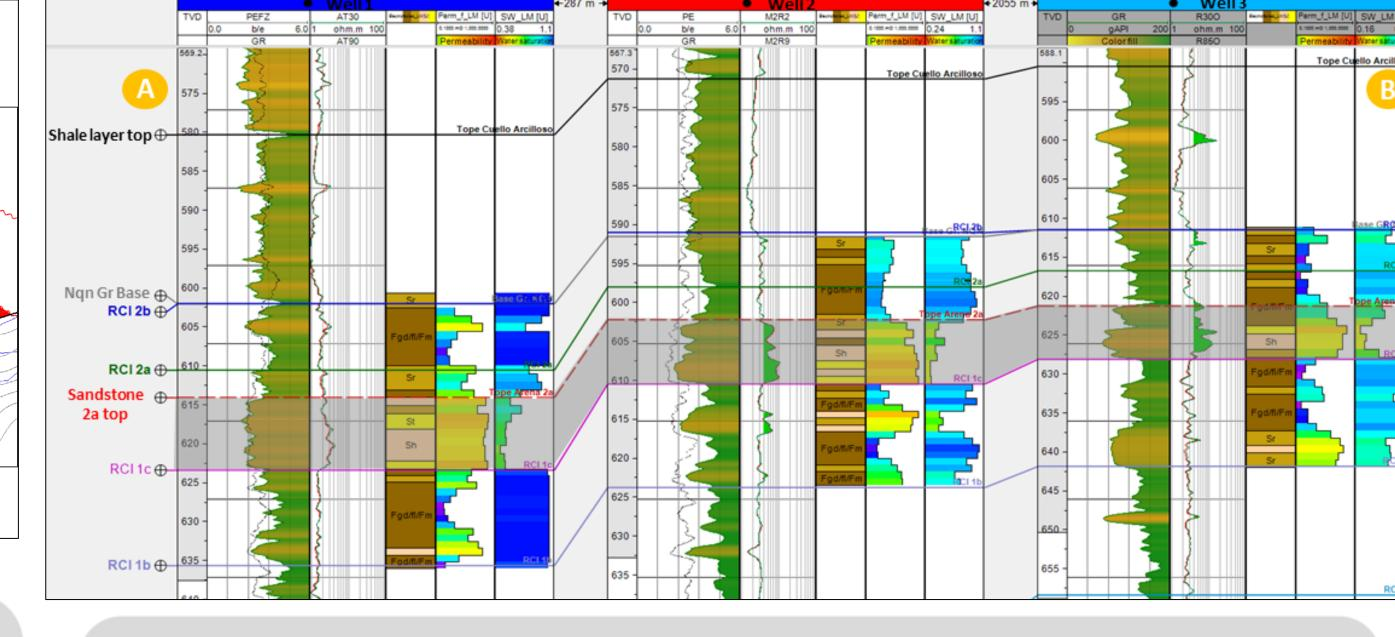
A static model was developed at first to identify the best zone to be navigated by the horizontal wells. The target in Block IV is the thickest sandy cycle of up to eight meters in thickness and the largest areal extent (cycle 2a). This cycle presents the best petrophysical properties in the three basal meters, which made it the target for navigation
