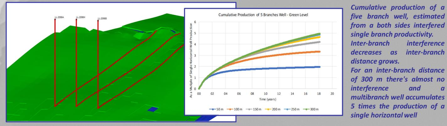
five branch well, estimated from a both sides interfered single branch productivity. interference Inter-branch decreases as inter-branch distance grows. For an inter-branch distance of 300 m there's almost no interference multibranch well accumulates 5 times the production of a
