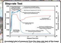
Copper Ridge in interval 3,695 - 3,945 ft PBTD. Inject Secondary fractures began to develop after pumping 36 BM and pressure had built to 2,301 psi. Pressure subsequently slowly increased to a maximum of 2,371 psi after injecting 392 BW, at which time the test concluded and the wellbore shut-in Pressure falloff was monitored for 6.8 hrs. after which i
