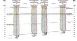
Stratigraphic cross section through the Knox Group shows thinning of lower Copper Ridge to the northeast
