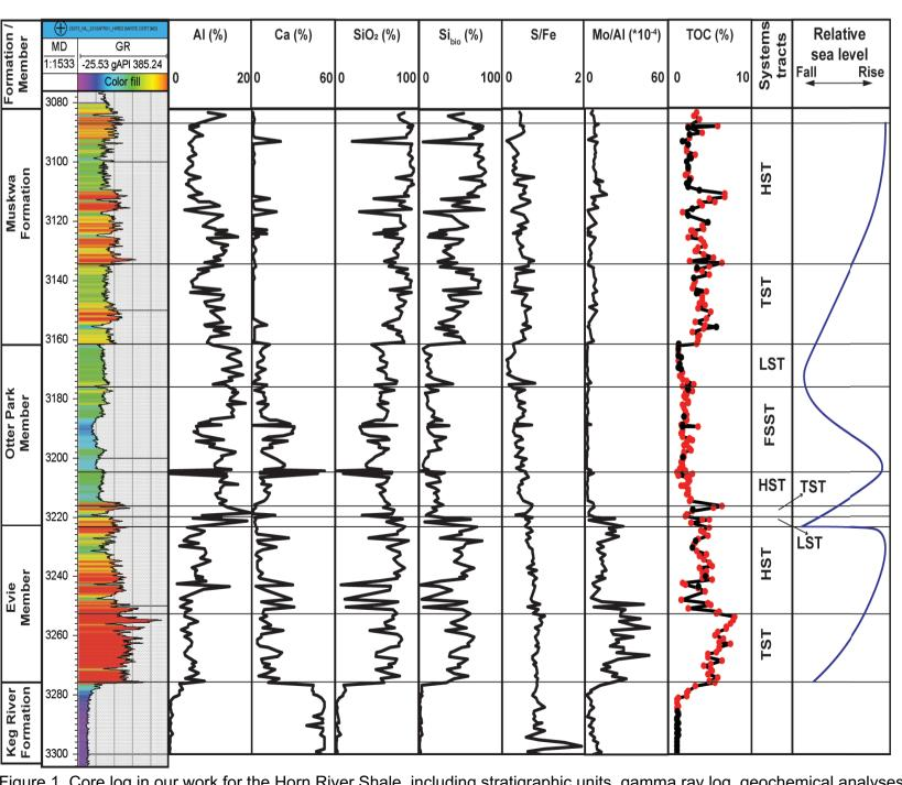
Figure 1. Core log in our work for the Horn River Shale, including stratigraphic units, gamma ray log, geochemical analyses (by ICP-MS and LECO analyses), and systems tracts distribution (sequence stratigraphy was based on Ayranci et al., 2018).
