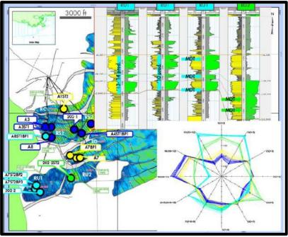
J2 sand structure map with geochemical fingerprinting using  $C_8$ - $C_{10}$  alkylbenzenes (MDGC).
