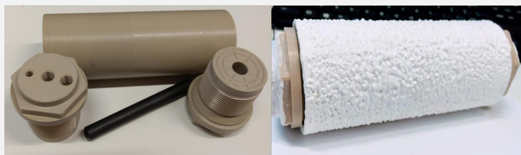
Figure 3. Core holder assembly and thermal insulation
