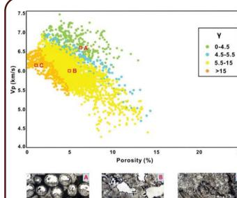
Velocity differs significantly at a given porosity due to different pore types, which can be explained by frame flexibility factor γ.
