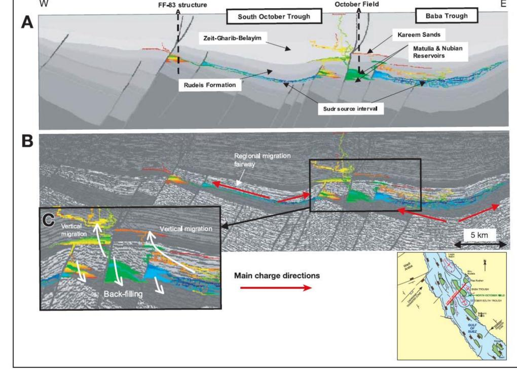
Migration pathways are color-coded according to their sequence. Blue is the earliest, then green, yellow and red. (A) Stratigraphy. (B) Stratigraphy superimposed on 2-D seismic section. (C) Main filling directions into the October Field. (Ghamri et al., 2002)
