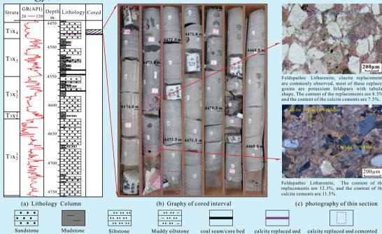
5. Well-tie section of tightly calcite replaced and cemented intervals in Xujiahe Formation, NE Sichuan Basin
