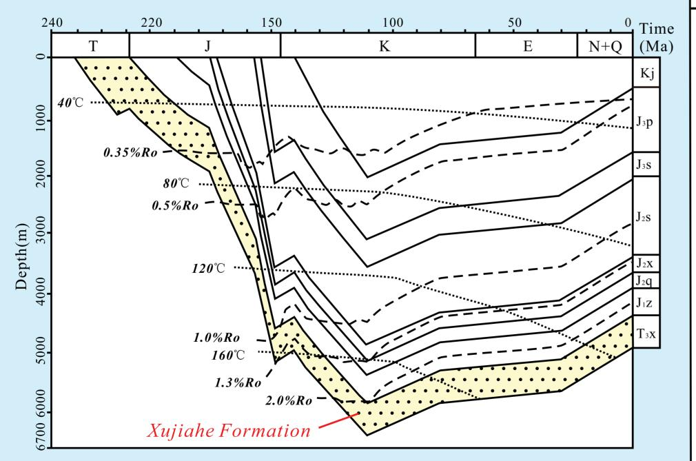
The burial and thermal history show that the maximum burial depth of T<sub>3</sub>X are reached 5800-6300 m during the period of Middle Crataceous, and the maximum geotempture was 180-220°C with a corresponding vitrinite reflectance (Ro%)≥2.0%.
