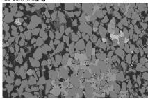
Scanning Electron Microscope (SEM) Backscattered Electron (BSE) image of sample from Paluxy formation with resolution of 1.13 µm.
