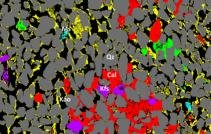
Segmented mineral map showing: Qz = Quartz; Kao = Kaolinite; Kfs = K-feldspar, Cal = Calcite; Ms = Muscovite, Sd = Siderite.
