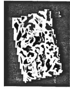
Figure 10: A vertical slice of the caliper cube highlighting areas where washouts have occurred. Light blue represents areas where the caliper reading is greater than nine inches and dark blue represents a caliper reading of less than nine inches. Note that the majority of washouts have occurred in the more friable Yates formation.
