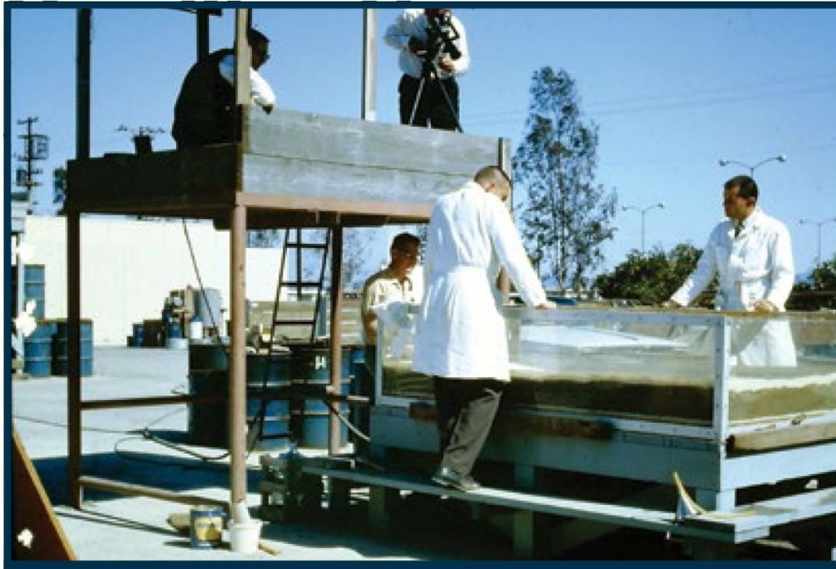
Figure 4. Manley Natland (with camera) filming the generation of turbidites in a flume at Union Oil Research Laboratory, Brea, Calif., January 1965. Photo courtesy of Martin Natland.
