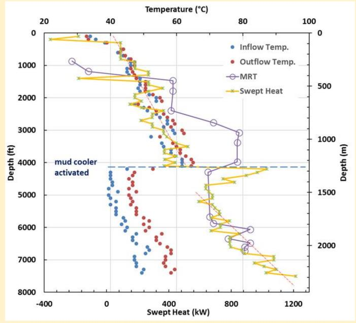
Drilling Indicators of Increasing Temperature with Depth
