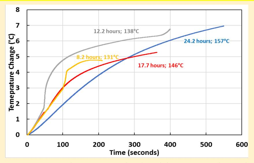
This response is attributed to radial temperature gradients in the rapidly heating hole, and mixing caused by the arrival of the probe
