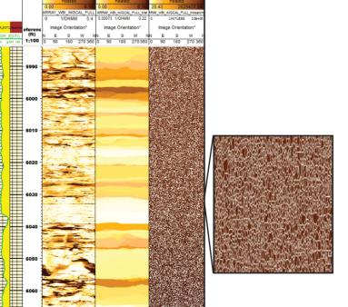
ABOVE: Examples of final Porotex results for two offset wells, X and Y, about 5 miles from each others, from West Texas. It is interesting to observe the variation in the heterogeneity distribution between the two wells but also along one single well. Also, there is a noticeable difference between the overall matrix porosity between the two wells
