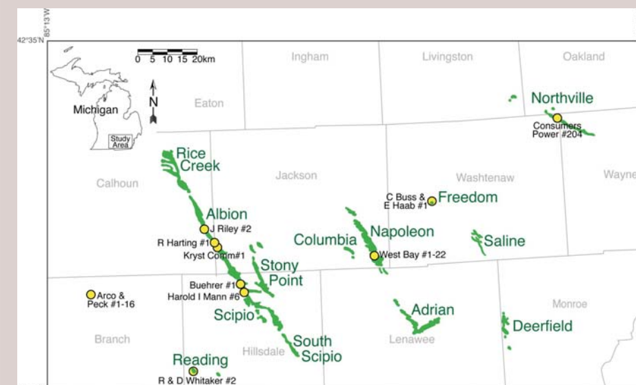
Figure 3. (Above) Fault-fracture dolomite petroleum reservoirs in the Trenton and Black River formations in southeastern Michigan are shown in green. Cores used in this study are yellow circles. Note the elongate NW-SE geometry and narrow width of the productive fields. Reservoir dolomites form along pre-existing brittle failure surfaces and are stratigraphically bound by tight host limestones distal from dolomitized zones. A seal is formed by the overlying cap dolomite and Utica Shale.
