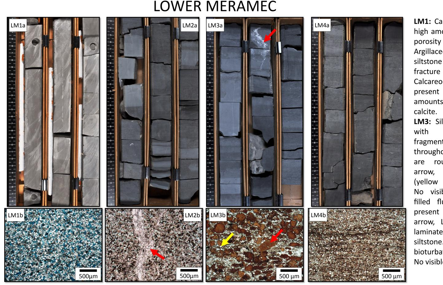
•Based on log and core data , the Upper and Lower Osage are dominated by chert-rich grainstones and packstones, while the Upper and Lower Meramec consist of argillaceous and calcareous siltstones. Calcite-healed fractures are common in carbonate-rich intervals.
