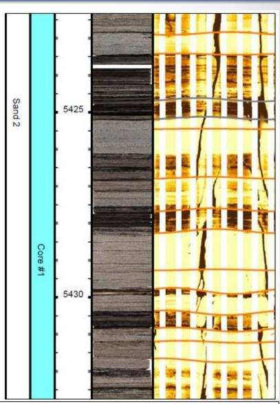
This series of fractures appears in the image logs in the Almond Formation reservoir. No fractures are present in the core
