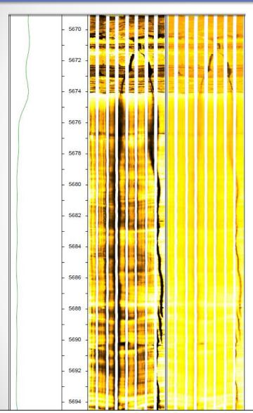
This ~20' fracture is the only one of it's size we've seen in image logs in the Trail section
