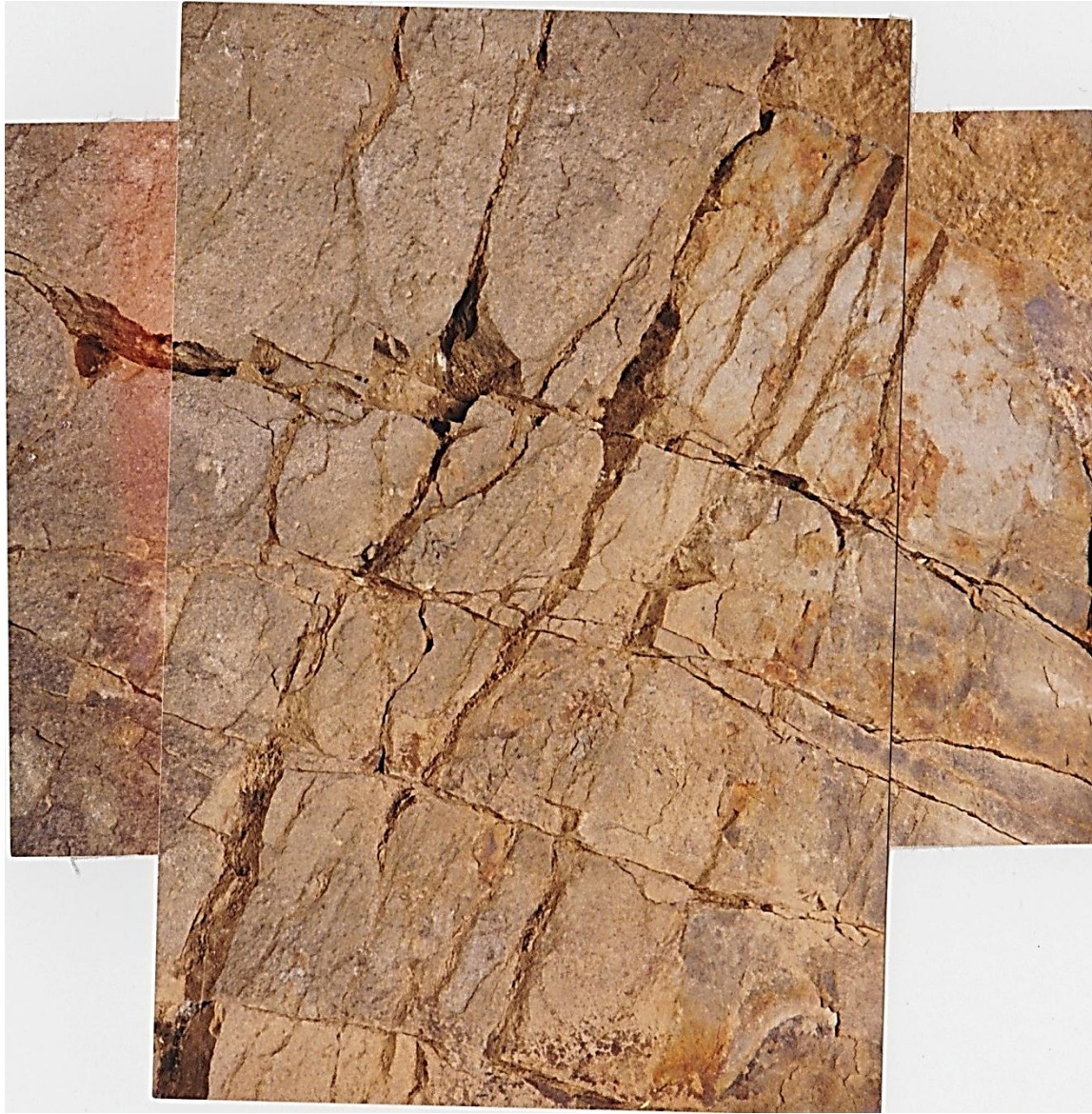
Fractured Permo-Triassic tuffaceous formation of the Choiyoi group. It is one of the main reservoirs in the Medanito field.
