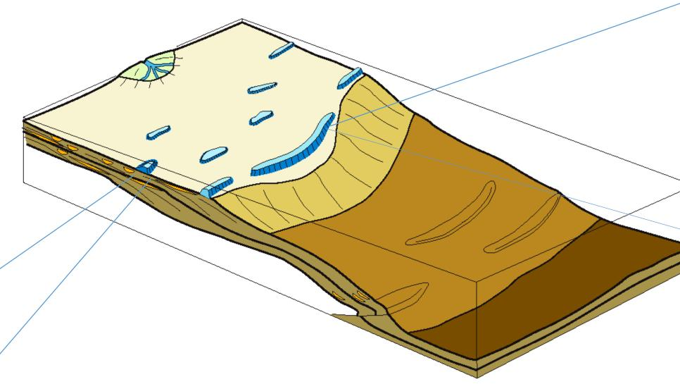
During Transgression & Rapid Sea Level Rises, Siliciclastic Shorelines Moved Landward & Carbonates Grew. Biggest Carbonate Buildups are on the Shelf Margin. Small Buildups on the Middle Shelf
