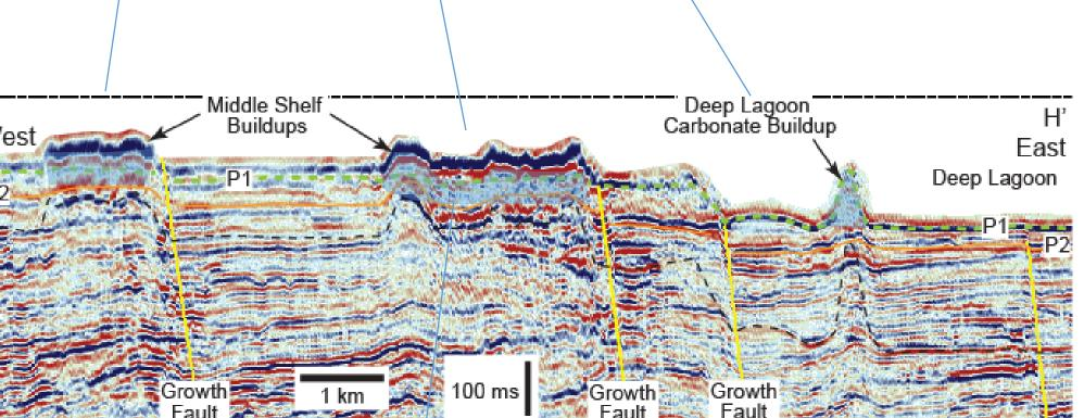
Shelf Interior Buildup on Upthrown Side of Fault
